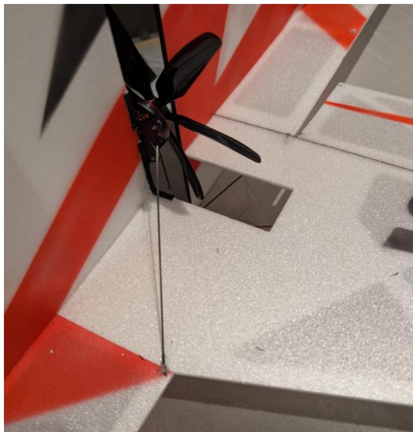
The approximate position of the balance point is at the leading edge of the propeller cutout.
